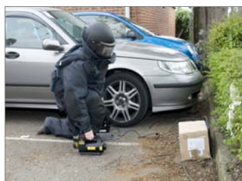
SCANWEDGE being set up to check a suspicious package in a carpark.
