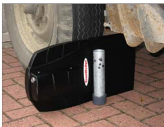
SCANWEDGE 2520 positioned on its side behind pipe bomb.
