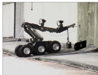
SCANWEDGE being positioned by ROV. Brackets available to adapt to all ROVs.
