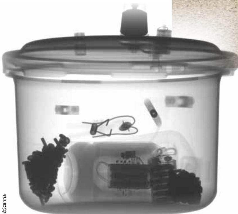
display crucial information regarding the functional IED components, allowing the operator to identify them by their shape, as well as revealing the locations of these component parts. This allows for a safe and successful disposal of the device.
