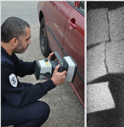
LEFT: MINI Z system scanning passenger door RIGHT: X-ray image of concealed currency
