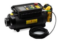
Scantrak is supplied with the Golden XR200 pulsed x-ray source with 2 x 18V Li-lon Batteries. We can also supply with alternative pulsed generator models -XR150/XRS-3/XRS4. The Scantrak imager is also available as an ICU upgrade for existing Scantrak customers to connect to their own Golden x-ray source or approved CP x-ray source.
